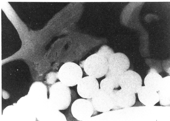
Figure 3 Microradiography from a group A specimen bead diameter 250–350 \mu\text{m} (X30). Underestimation of porosity (spaces without metal) and overestimation of the area covered by bone are apparent when compared with Fig. 2.
